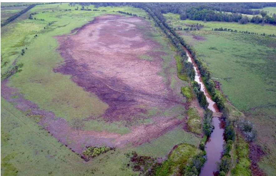
Photo: Drainage channel and acid soil scald at Yerbury Scald (T. Tucker WRL)
