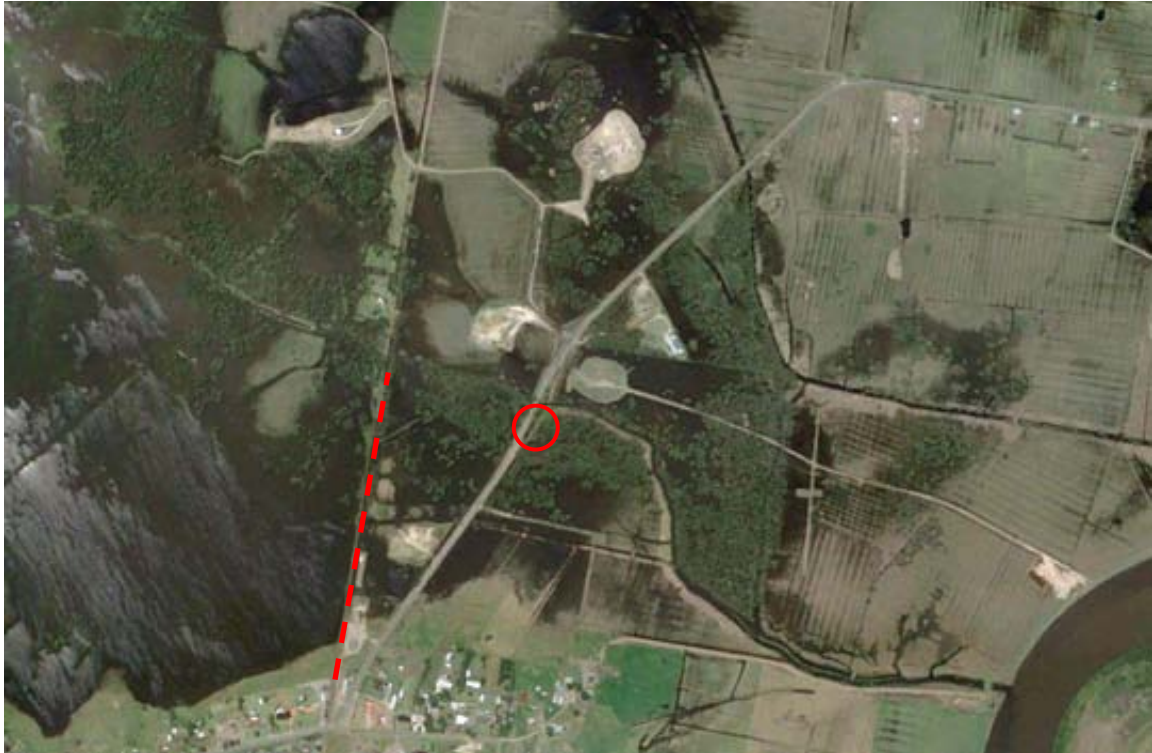
Figure 8.4: Removed section of pipeline, and modified Woodberry Road cross-section for numerical model scenario (Background image: Google Earth)
