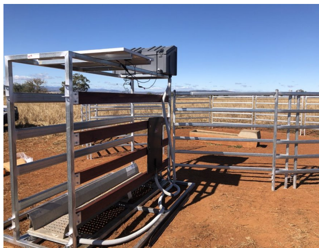
IMAGE 1: Walk over Weigh (WoW) set-up showing the panel reader on the right side, solar panels and box for telemetry equipment on the top.
