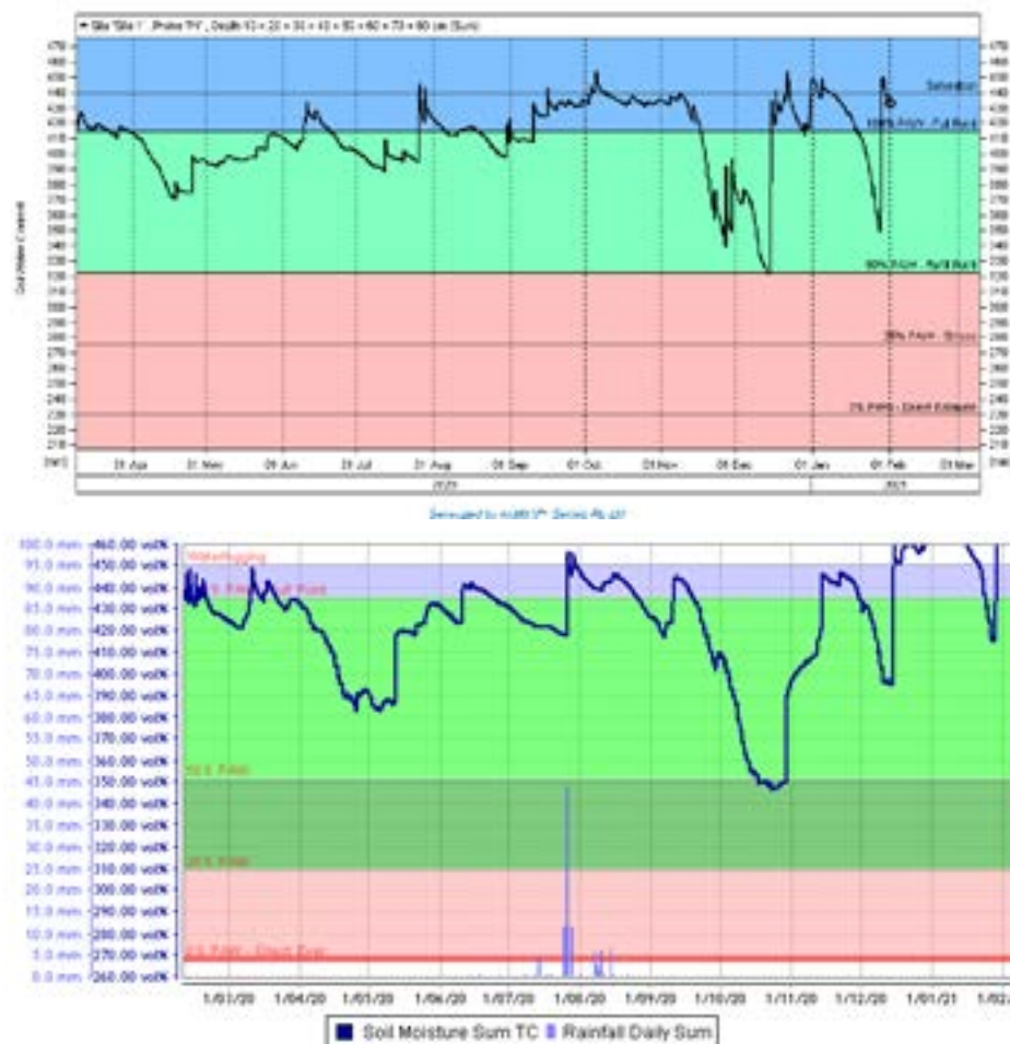
← Figure 1- Kwong Flat soil moisture graph shows that Adam maintained RAW during the Nov-Dec dry-spell then waited for forecasted rainfall mid-December to lift soil moisture. Decline was again addressed by forecasted rainfall in late January.
