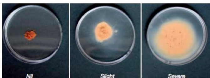
Figure 4: Examples of degrees of dispersion of soil aggregates after 24 hours in water.
