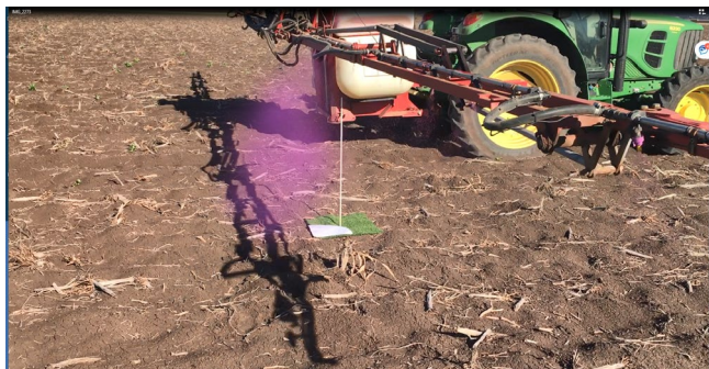
Figure 1. Spray nozzle activates in the vicinity of piece of astro turf that was previously mapped using a drone.
