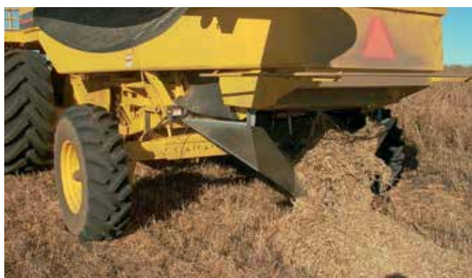
A header with a chute attached that is used to make narrow windrows for burning.
