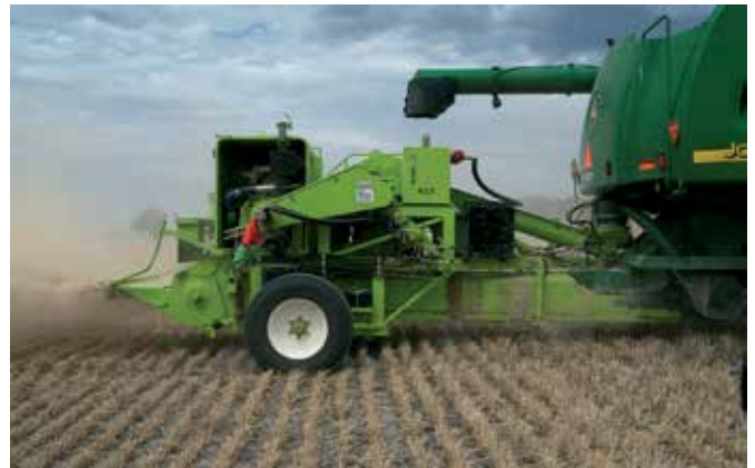
A Harrington Seed Destructor reducing ryegrass seed numbers in Western Australia.
