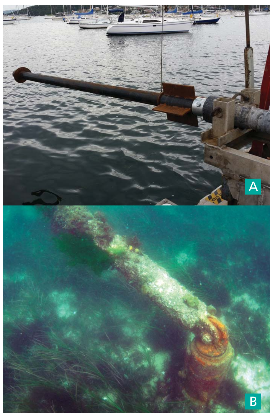
Figure 2 [A] Seagrass friendly mooring ready to be installed at Belmont, Lake Macquarie [Photo Des Maslen]; [B] seagrass friendly mooring at Shoal Bay [Photo Bill Gladstone].
