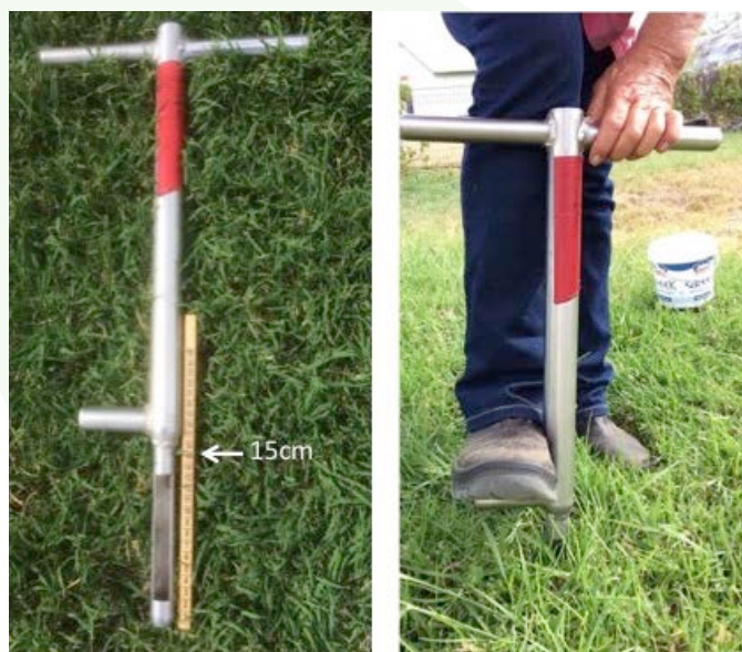
Figure 1: A soil corer and appropriate use.
