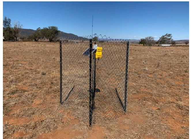
IMAGE 3: Soil moisture probe on site at Manilla, NSW.
