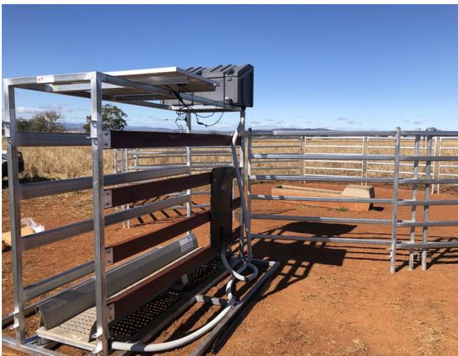
*IMAGE 1: Walk over Weigh (WoW) set-up around a water point at the Lockrey's in Manilla, NSW.*
