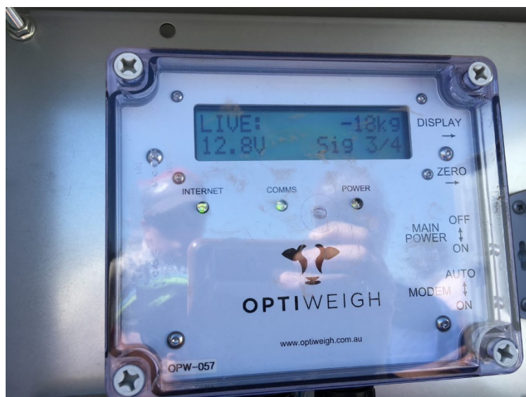
Display on the Optiweigh unit showing a -18kg tare weight.
