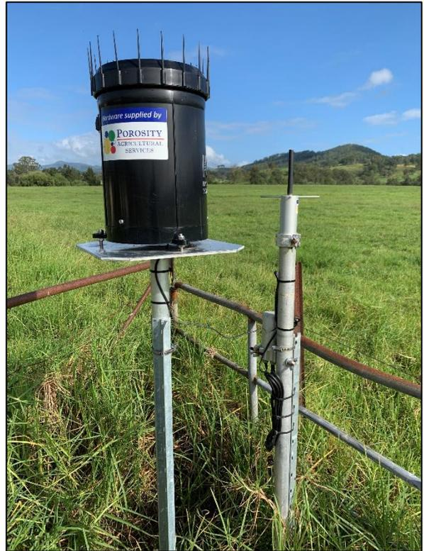
*Figure 3. The tipping bucket rain-gauge on both farms has been replaced with higher quality units connected to the existing data logger and telemetry.*
