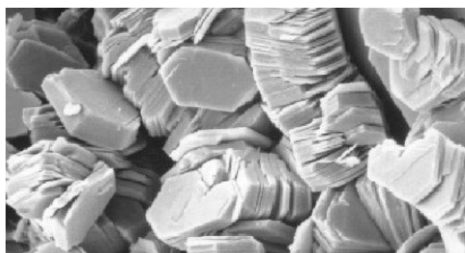
Figure 1: Electron microscope image of kaolinite clay layers
